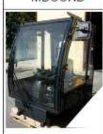
The forklifts of the Series Elephant 35/20, 25, 30 e 35 can be ordered with a high visibility cabin made of a steel frame and special glass. Thanks to the cabin, maximum comfort is granted to the operator also with bad weather.
