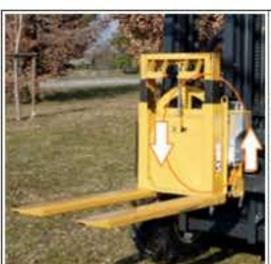
All the fork-lifts of the Series Elephant, thanks to the coupling type FEM2, can be equipped of a bin rotator operated hydraulically from the seat.
